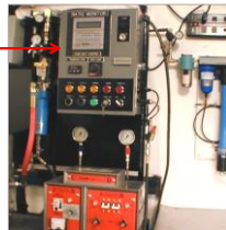
Aftermarket flow ratio, usage totalizer, and temperature monitor system with auto shut-off added to standard proportioning equipment.
