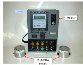
These are the two main components of a temperature and ratio monitoring system.
