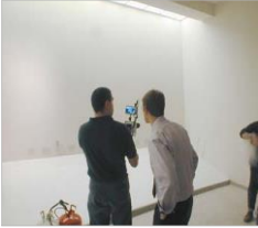
Infrared QC of foamed-in-place insulation behind 1" plaster – effective year-round (240F)
