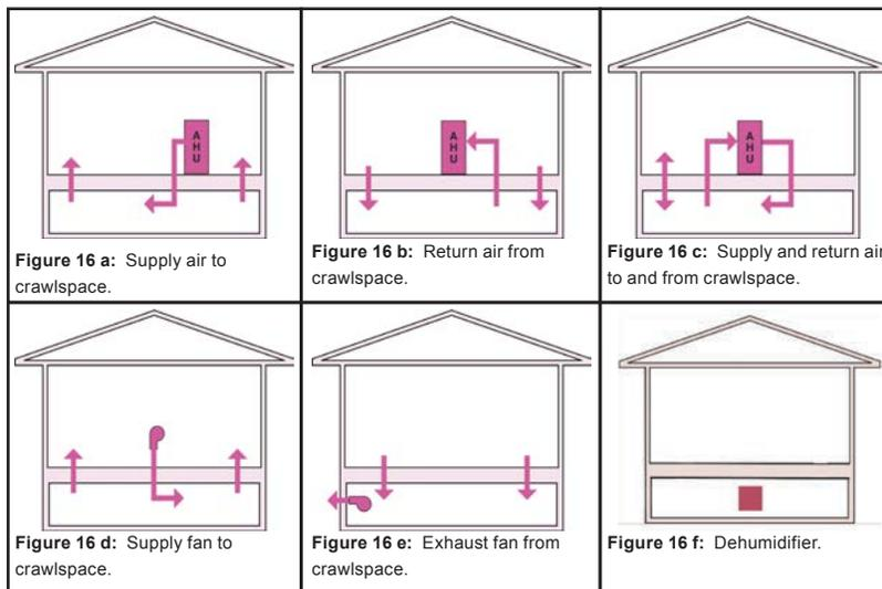
**Figure 16 a:** Supply air to crawlspace.
