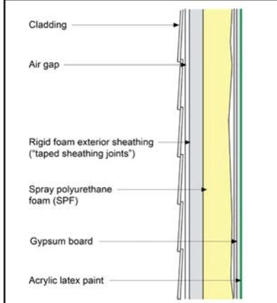
Notes: High density closed cell foam can be used in all IECC Climate Zones. Where low density open cell foam can be used the thickness or thermal resistance of the rigid foam exterior sheathing is specified by the International Residential Code (IRC) based on Climate Zone and the thickness of the wall framing.
