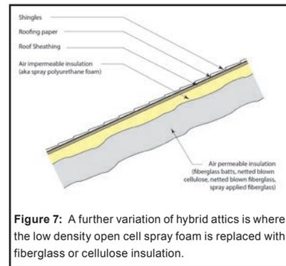
**Figure 7:** A further variation of hybrid attics is where the low density open cell spray foam is replaced with fiberglass or cellulose insulation.
