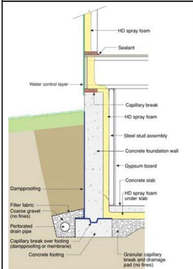
**Figure 11b:** Spray foam insulation can be directly applied to the interior of concrete foundation walls and under basement floor slabs.
