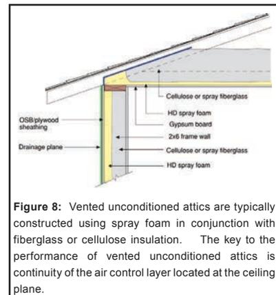
**Figure 8:** Vented unconditioned attics are typically constructed using spray foam in conjunction with fiberglass or cellulose insulation. The key to the performance of vented unconditioned attics is continuity of the air control layer located at the ceiling plane.
