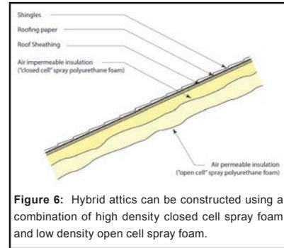
**Figure 6:** Hybrid attics can be constructed using a combination of high density closed cell spray foam and low density open cell spray foam.
