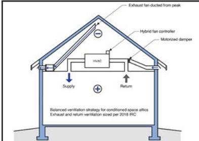
**Figure 10:** The best way to remove moisture from the attic space is to provide air change. Air is exhausted from the peak of the attic using an exhaust fan ducted to the exterior.
