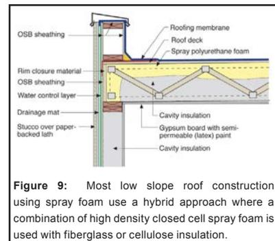
**Figure 9:** Most low slope roof construction using spray foam use a hybrid approach where a combination of high density closed cell spray foam is used with fiberglass or cellulose insulation.
