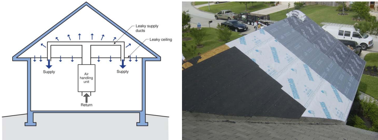
Figure 13. Air leakage communication from unvented attic to main space (left); Houston-area roof underlayment study (right)
