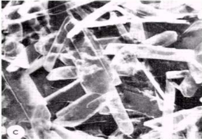
Figure 1c. Gypsum, hydrated from plaster of paris and water, porosity 30 per cent.
