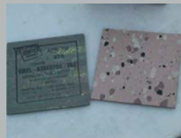
Vinyl asbestos flooring
